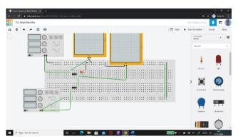
Fig 6: Circuit of Full Wave Rectifier in Tinkercad before simulation
