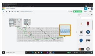
Fig 5: Circuit of positive peak clipper in Tinkercad
