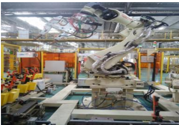
Fig. 1: Spot welding robot
