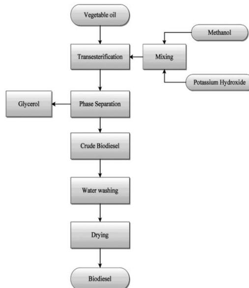
**Fig. 2 Flow chart for production of Biodiesel**
