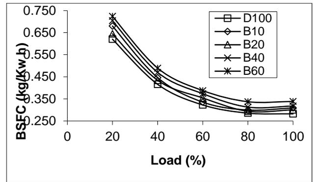
Figure 4 Effect of biodiesel quantity on BSFC
