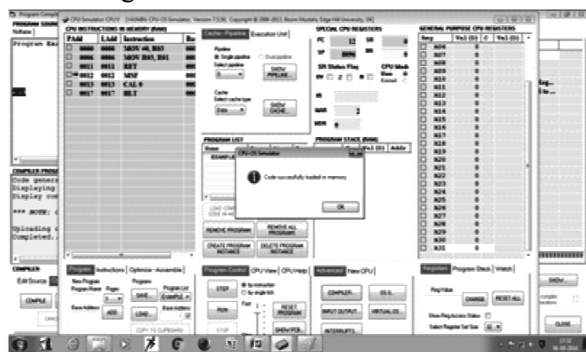
Fig.4: Loading machine language program in main memory of CPU-OS Simulator
