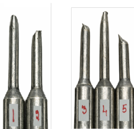
Fig 2. Fatigue Test Specimens, a) Un-peened Al and AMMC, b) Laser Peened AMMCs
