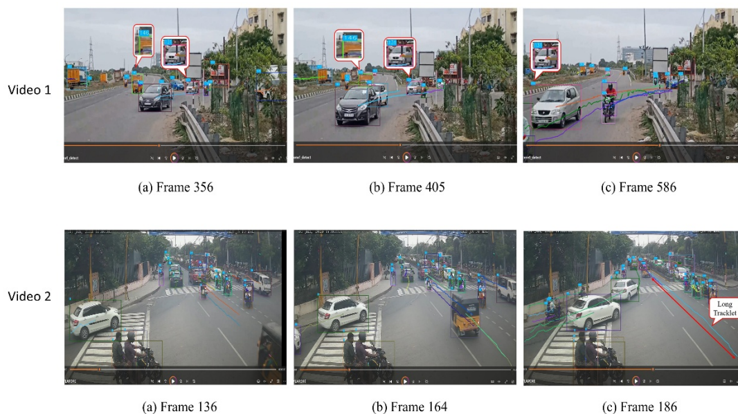
Fig 6. Multi-vehicle tracking on Video 1 and Video 2 with unique ID using Enhanced DETR-ByteTrack algorithm
