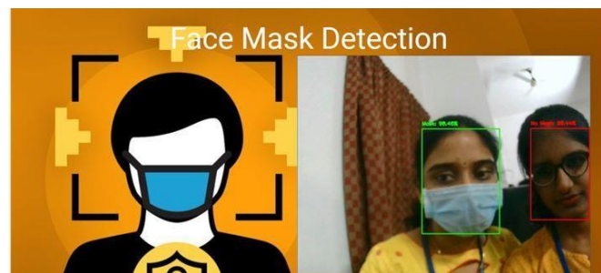
Fig 7. Proposed model identifying 2 people staring at the screen, of which one is wearing a mask and highlighted by green color and the other with red color who is not wearing a mask
