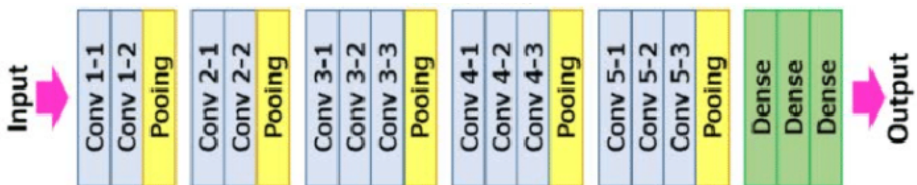
Fig 3. Architecture of VGG 16
