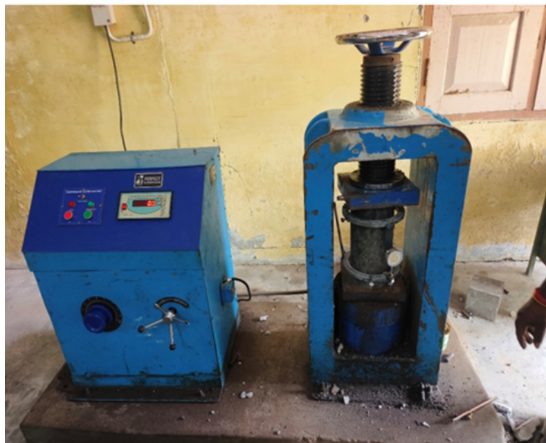
Fig 4. Modulus of Elasticity Test Setup
