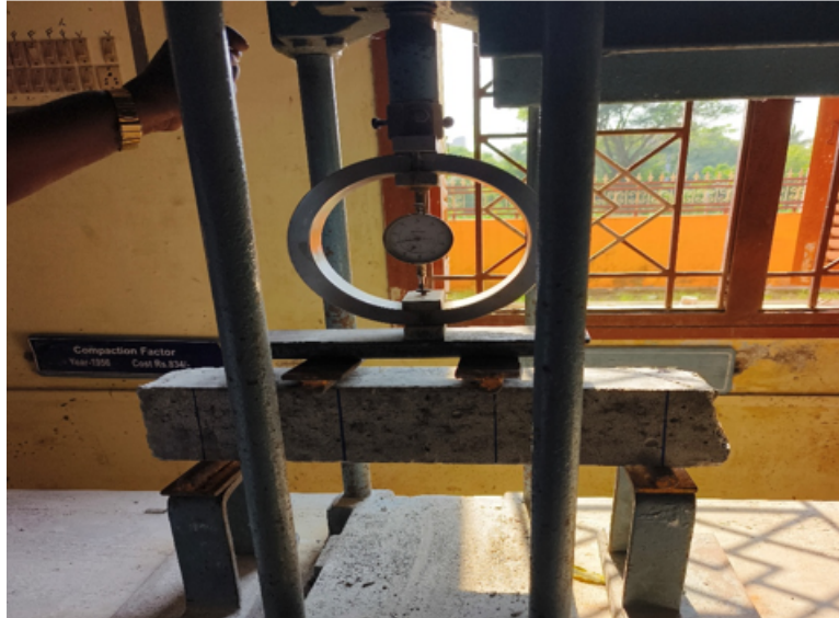
Fig 3. Flexural Strength Test Setup
