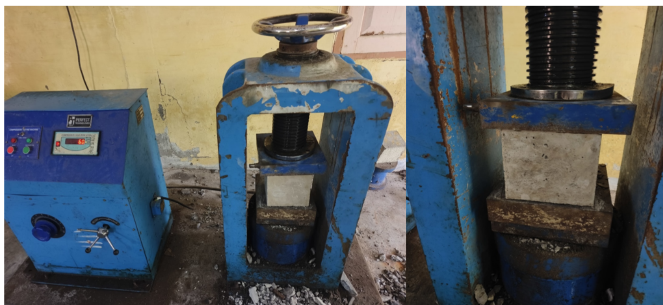
Fig 2. Compressive Strength Test Setup
