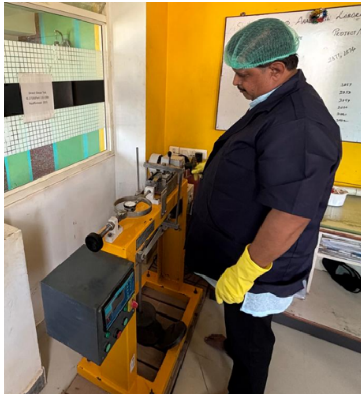
Fig 8. Direct Shear Strength Test
