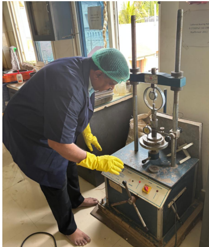
Fig 9. Unconfined Compressive Strength Test
