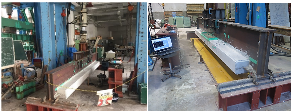
Fig 7. Data acquisition of post-damage state of the girder
