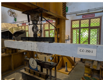
Fig 2. Loading Setup for the Beams
