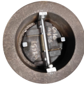
Fig 1. Dual Plate Check Valve with Helical Torsion Spring. The valve used in the problem under study for the industrial application is utilizing single helical torsion spring due to smaller size of the valve. The problem under study is focusing on identifying optimum value of spring diameter that give higher life cycle.
