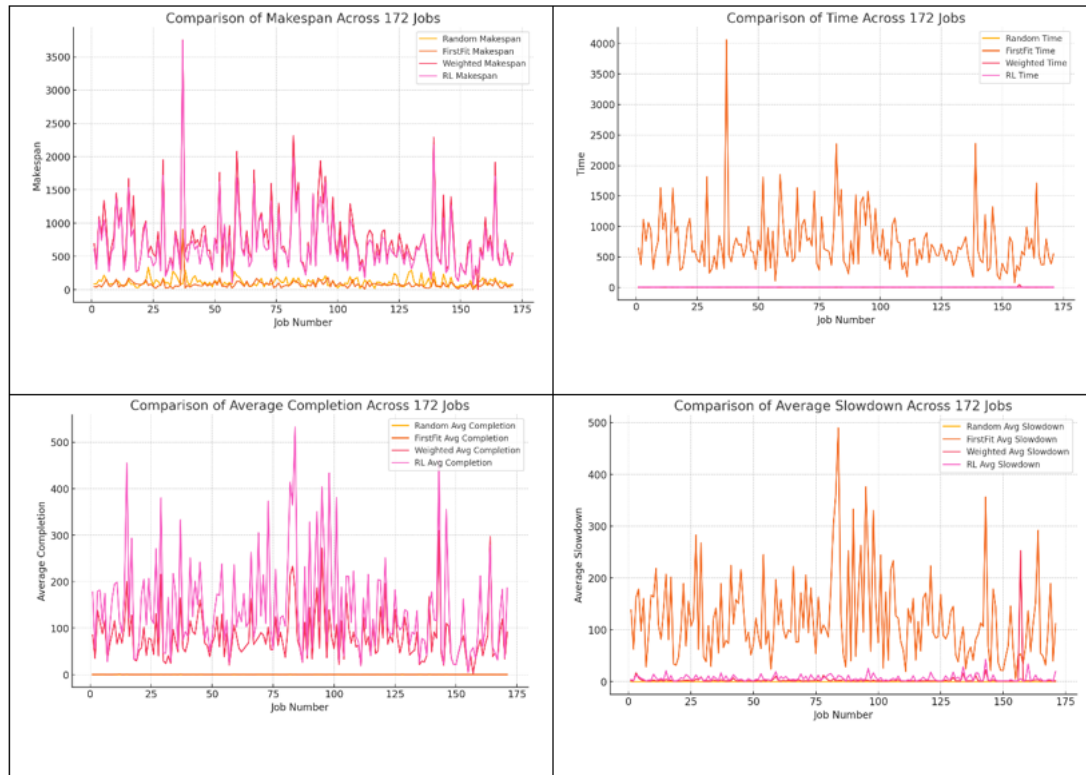
Fig 3. Comparison of Makespan, Time, Average Completion and average Slowdown across four algorithms for 172 Jobs
