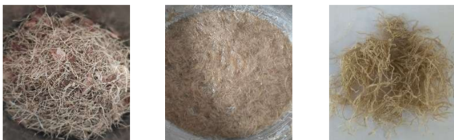
Fig 2. Fibres are extracted from ACF roots by the method of water retting process
