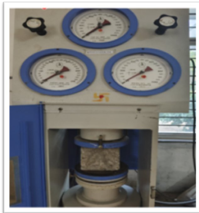
Fig 2. Compressive Strength Test Setup
