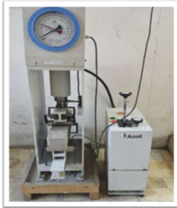
Fig 3. Flexural Strength Test Setup
