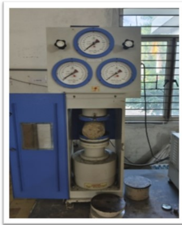
Fig 4. Splitting Tensile Strength Test Setup
