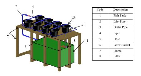
Fig 1. The design of the experimental set-up
