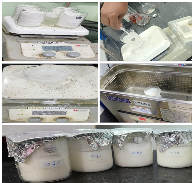
Fig 1. Steps of Nanoparticle Enhanced PCM preparation. a. Melting of Paraffin Wax, b. Dispersion of Nanoparticles in the Paraffin Wax, c. Stirring Process, d. Ultra-sonification Process, e. Prepared Samples
