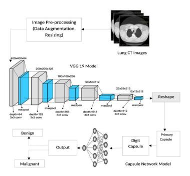
Fig 5. The architecture of the VggCapNet
