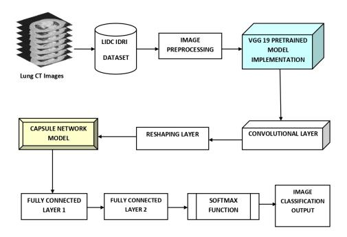
Fig 3. VggCapNet Model using VGG 19 and Capsule Network
