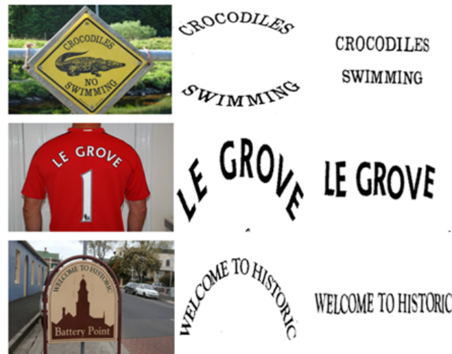
Fig 4. The rectification results of the proposed method; first column shows the original curved scene text images from CUTE 80 dataset. Second column shows the binarized images and the third column shows the rectified text using B-spline curve fitting.
