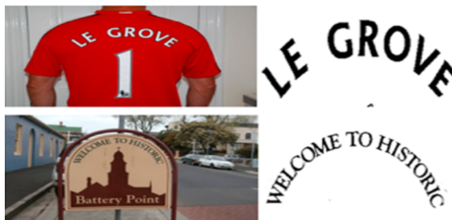
Fig 3. The sample results of binarization on scene text images of CUTE80 dataset. The first column shows the original scene text images and second column shows the binarized curved text.
