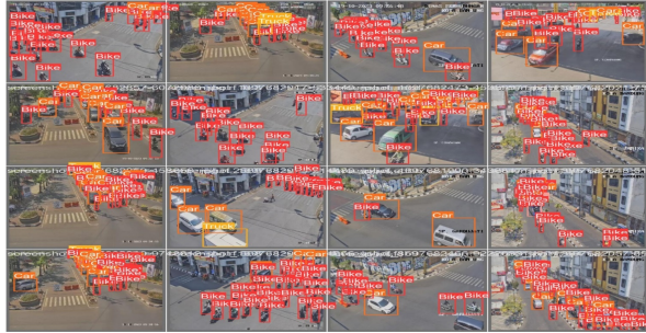
Fig 6. Predicted Results for all four classes (bike, Bus, Car and truck) and background for the fine tune model for test dataset
