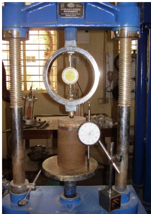
Fig 2. Unconfined Compressive Strength Test Set up
