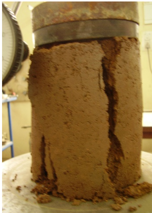
Fig 3. Shear failure of soil specimen stabilized with Wollostonite
