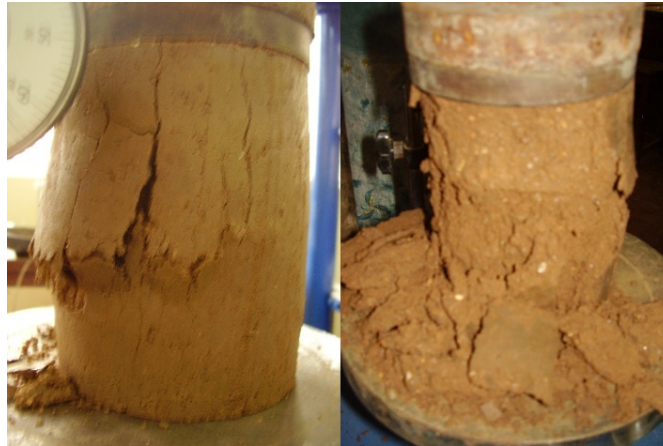
Fig 4. Progressive shear failure of soil specimen stabilized with Wollastonite
