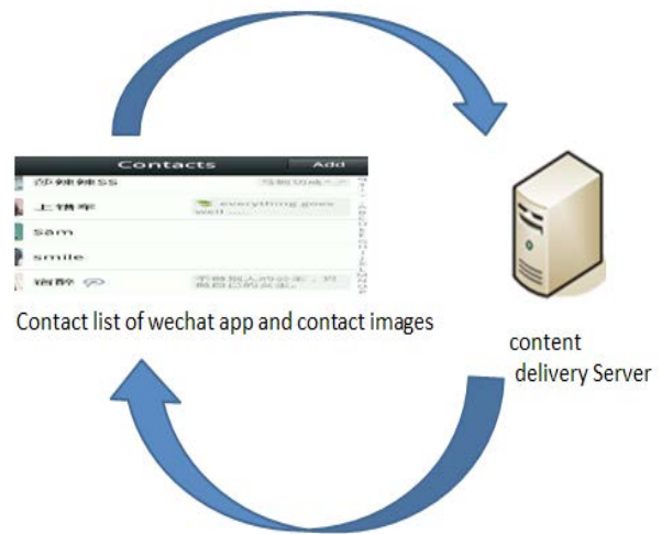
Figure 3. We chat display Contact list small images individually loading images in app increase HTTP request.
