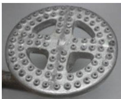
Figure 5. Conventional “concentric-cross” free flame self-aspirating burner for industrial cooking.
