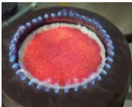
Figure 4. Porous and swirl burner working coupled.
