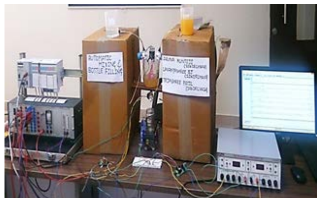
Figure 8. Hardware setup for the PLC control.
