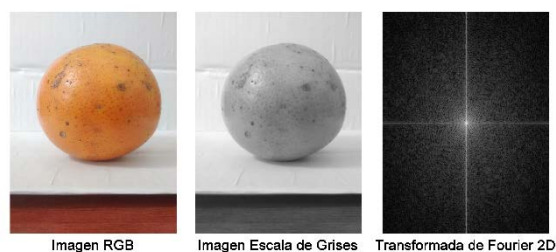
Figure 2. RGB, gray scale and frequency representation of a C. Tangelo fruit image.
