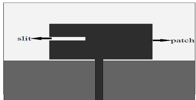
Figure 2. Notching slit in rectangular patch micro strip antenna.
