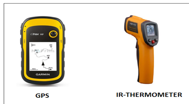
Figure 2. Equipment used in the field measurement of LST.
