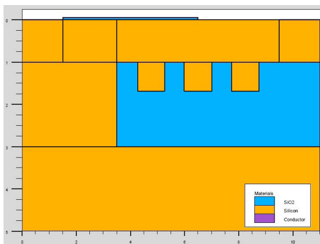
Figure 3. LDMOS device structure from process simulation
