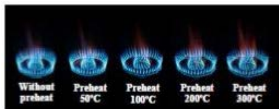
Figure 2. Effect of air preheating on structure of the flame at q=8.41\text{kW}^{18} .
