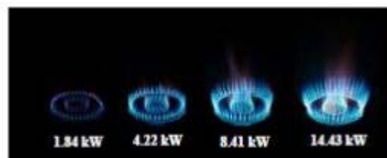
Figure 1. Effect of the heat input on the structure of the flame 18 .
