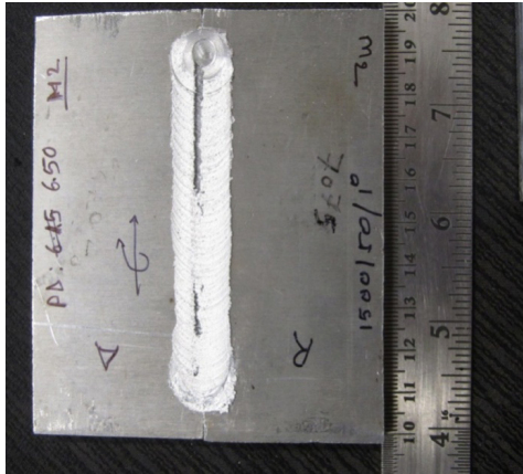
Figure 7. Test coupon welded at 1^\circ tool tilt angle.
