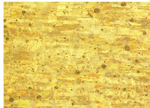
Figure 8 (d). Heat affected zone (200X).
