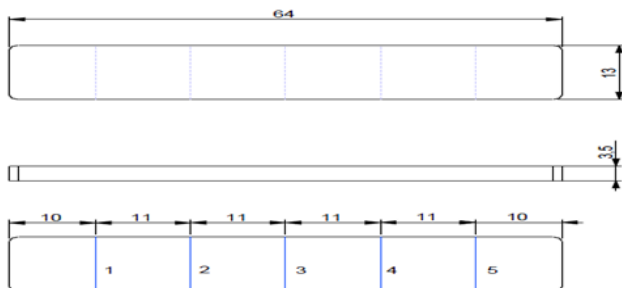
Figure 2. Specimen dimensions for shrinkage (ASTM D638).
