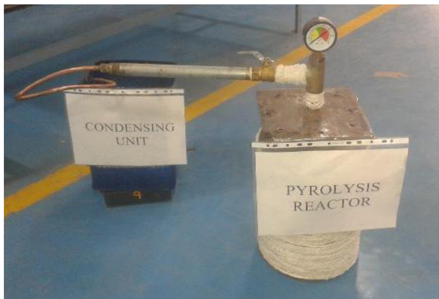
Figure 2. Actual picture of Pyrolysis reactor with its Condensing unit.
