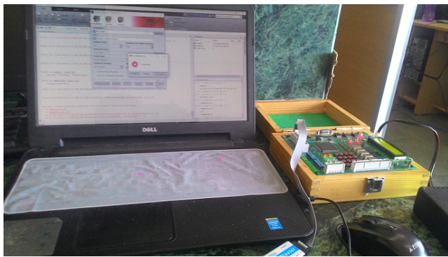
Figure 9. Hardware Cosimulation on Xilinx Spartan 3 Protoboard XC 3S 400board.
