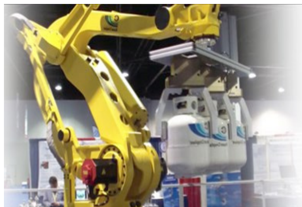
Figure 2. Robot for lifting the cylinders using grippers.
