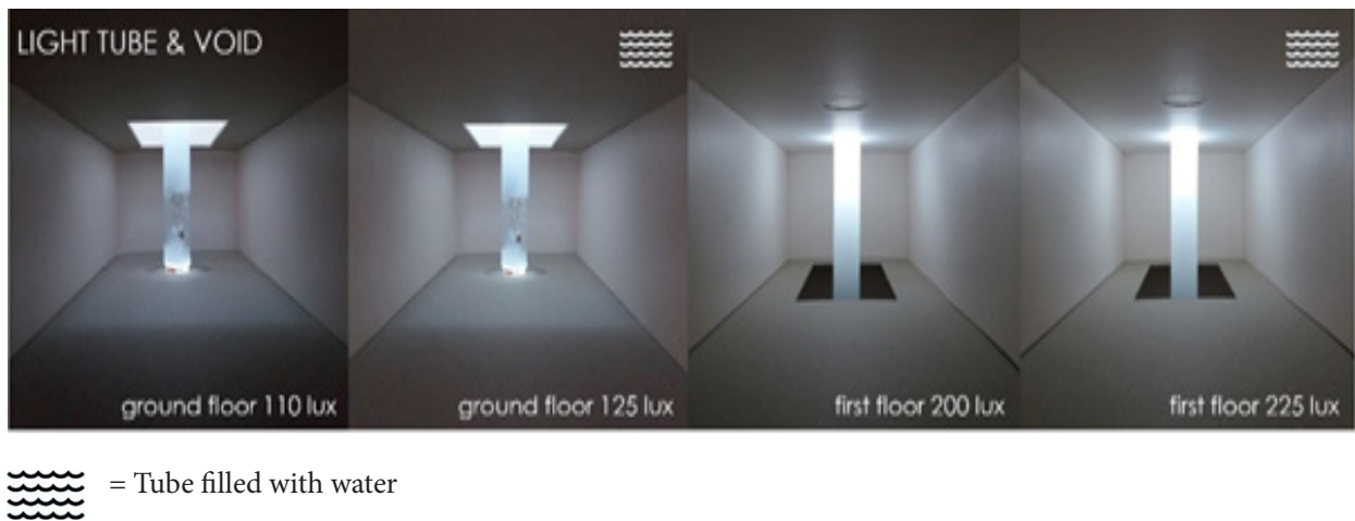
Figure 8. Void will increase the light intensity at the ground floor.
