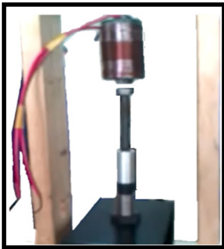
Figure 2. A single axis magnetic bearing system showing the magnetic coil, levitated steel bolt and eddy current position sensor.
