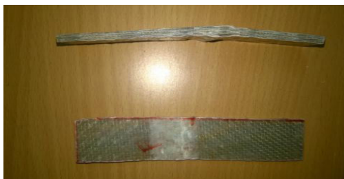
Figure 10. GABGRP (Al mesh) hybrid after flexural test (no de-lamination observed).
