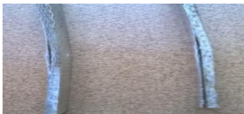
Figure 9. De-lamination of GABGRP (Al foil) hybrid after flexural test.
