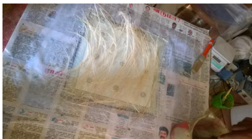
Figure 2. Hand layup process.
