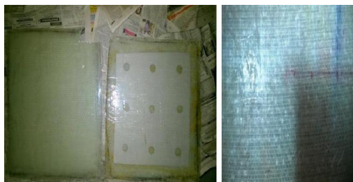
Figure 3. Final fabricated GFRP, GABRP (with aluminium foil) and GABGRP (with aluminium wire mesh).
