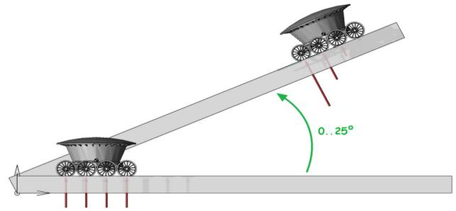
Figure 7. Initial and final position during visualization of Lunokhod-1 locomotion process modeling.
