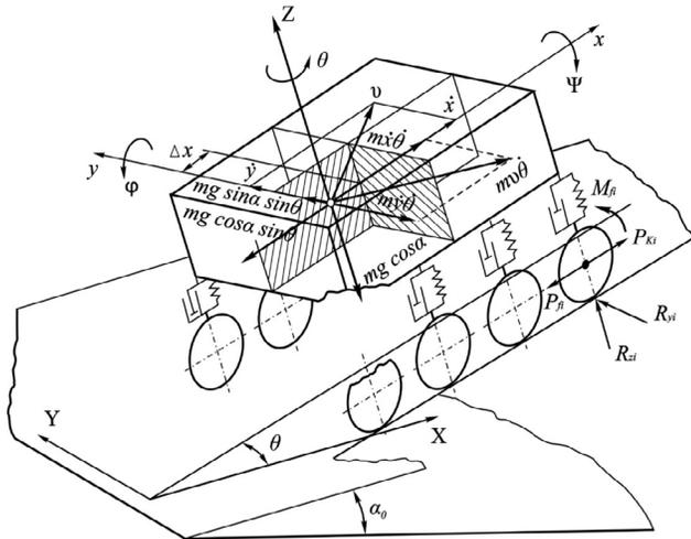
**Figure 2.** Calculated dynamic diagram of lunar rover with 8x8 wheel configuration and independent elastic wheel suspension.
