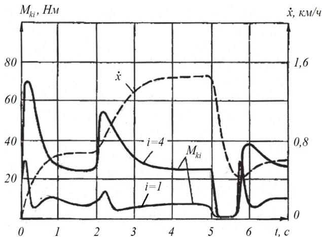
**Figure 6.** The results of modeling the dynamic loading of the motorized wheel drives –for the front and rear wheels during the ascent at  $\alpha = 10^\circ$ .
