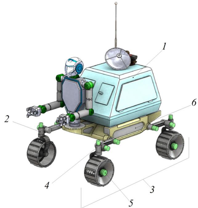
**Figure 1.** The components of Cosmonaut Assistant robotic system: 1 - container with detachable equipment; 2 - locomotion module; 3 - locomotion system; 4- two-lever walking mechanism; 5 - motorized wheel; 6 - locomotion system frame.
