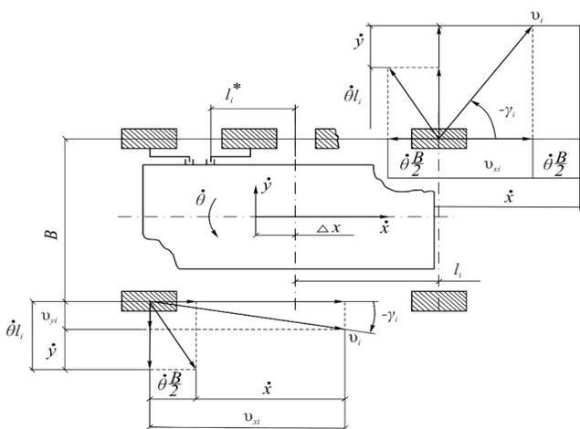
**Figure 3.** The  $i$ -th wheel velocity calculation scheme:  $O_1$  - the chassis geometric center projection on the supporting plane,  $O$  - lunar rover center of gravity projection.
