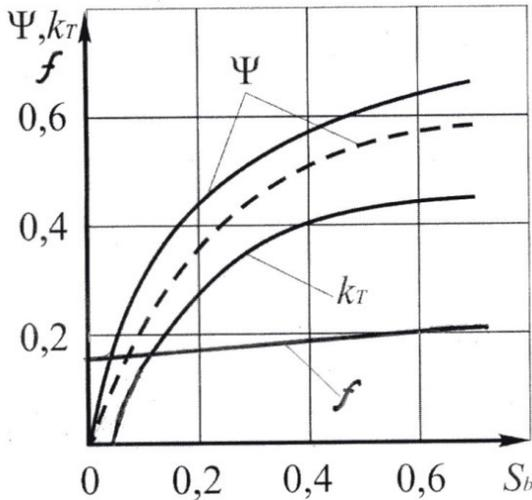
**Figure 5.** View of generalized frequency responses  $\Psi(S_b)$ ,  $f(S_b)$  during testing the Lunokhod-1 wheel on quartz sand (dashed line - during the Moon’s gravity simulation).
