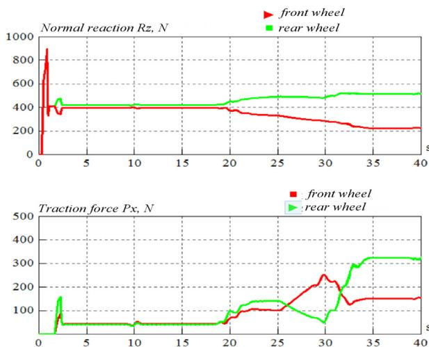
**Figure 10.** The results of simulating the locomotion system traveling on a flat and sloping surface with regard to the developed soil model.
