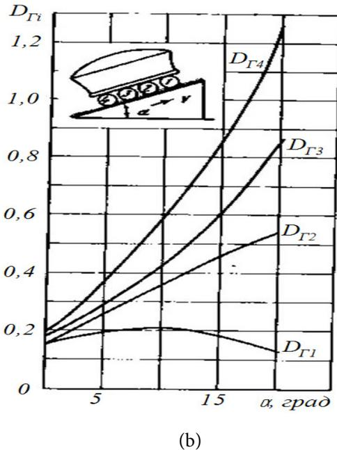
Figure 8. Comparison of dependency of the motorized wheel load factors on the angle of ascending: a - object-oriented modeling results; b - results of Lunokhod-1 experimental investigations.
