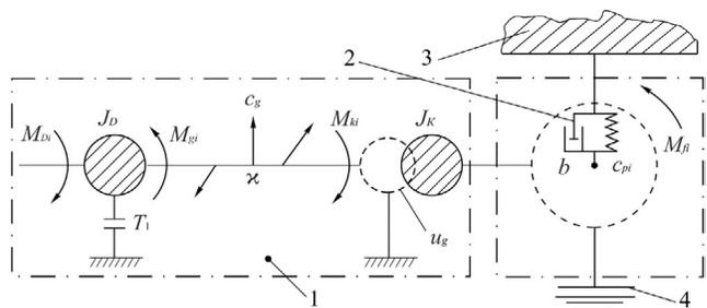
**Figure 4.** Calculated dynamic diagram of  $i$ -th motorized wheel 1 - electro-mechanical drive; 2 - suspension; 3 - spring-suspended section, 4 - conventional friction clutch connecting the wheel rim with the ground.
