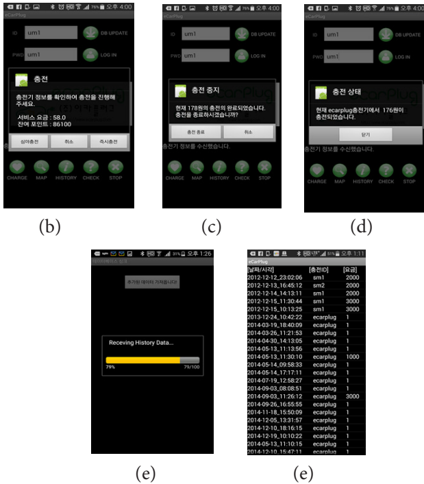
Figure 14. Smart phone interface screens for the proposed charging system (a) Locations of available charging stations (b) Charging start screen (c) Charging stop screen (d) Current charging state (e) Communication with service server (f) Data received from service server.
