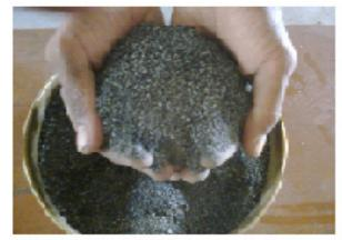
Figure 3. Pulverized burned LDPE fine aggregate.
