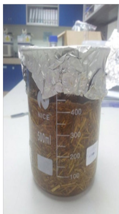
Figure 2. NaOH pretreatment of rice straw
