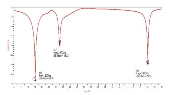
**Figure 6.** S-Parameter calculation of proposed coax fed MIMO antenna at port-2.
