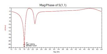
**Figure 3.** S-Parameter calculation of proposed antenna with single G-shape structure.
