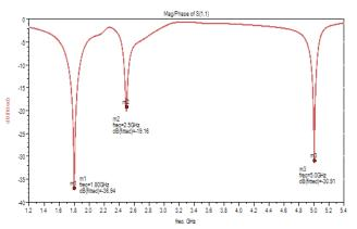
**Figure 5.** S-Parameter calculation of proposed coax fed MIMO antenna at port-1.
