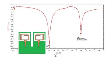
**Figure 4.** S-Parameter calculation of proposed MIMO antenna with out L-slot (**a**) at port-1 and (**b**) at port-2.
