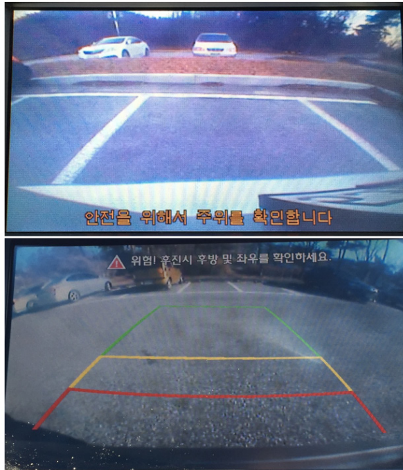
Figure 6. Example of parking assistant function display without and with guidelines.
