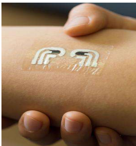
Figure 2. Tattoo type glucometer.
