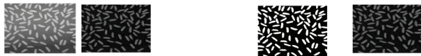
a) GrayScaleImage b) background removed image c) Image Binarization d) Filtered Image
