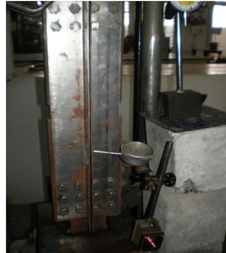
Figure 4. Experimental setup for double angle specimen connected to same side of the gusset plate ( t = 3\text{mm} ).
