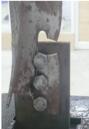
Figure 11. Mode of failure for single plain angle specimen (Block shear failure) (t = 3mm).
