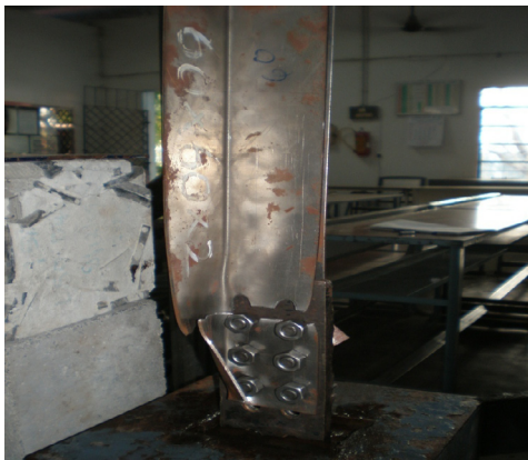
Figure 12. Mode of failure for double plain angle specimen connected to opposite side of gusset plate (Net section failure) (t = 2mm).
