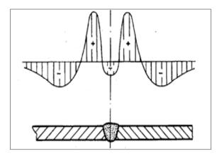
Figure 2. Residual stress distributions in butt weld.
