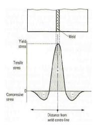
**Figure 3.** Types of residual stress in butt weld.
