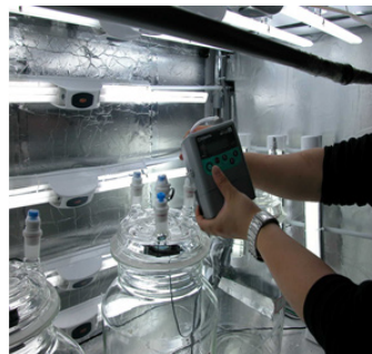
Figure 2. Measuring formaldehyde concentration using air bag.
