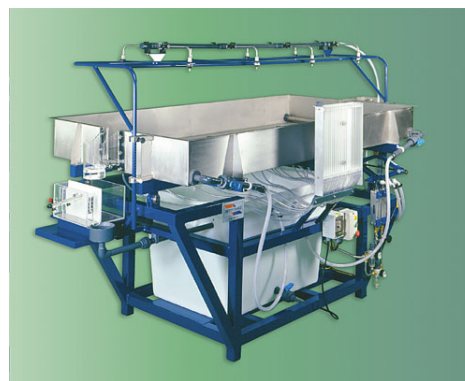
Figure 1. S-12 MKII-50 Advanced Hydrologic Systems (Rainfall Simulator).
